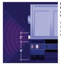
It is recommended that Grote WorkShield lamps are mounted at a height range of 48" to 72" off the ground.
