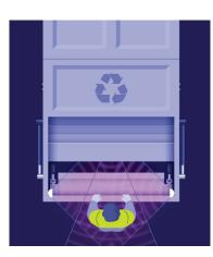
For applications which commonly have work taking place behind the vehicle, like on recycling trucks or tow trucks, we recommend two Grote WorkShield units be installed pointing inward to the center of the back of the vehicle.
