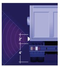
It is recommended that Grote WorkShield lamps are mounted at a height range of 48" to 72" off the ground.
