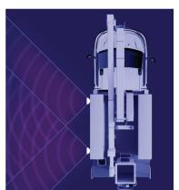
Service trucks or boom trucks may consider mounting the lamps at two locations on the vehicle so they converge at the center point and ensure maximum coverage and illumination of the work zone.
