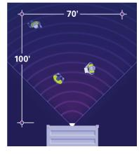
Grote WorkShield lamps create a triangular work zone that is approximately 3,000 square feet in size. It is important to ensure that the lamps are mounted so that workers (and high visibility materials) are operating in the center of this work zone. This will ensure maximum visibility.
